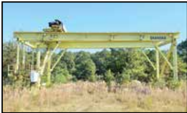
25-Ton Gantry Bridge Crane
